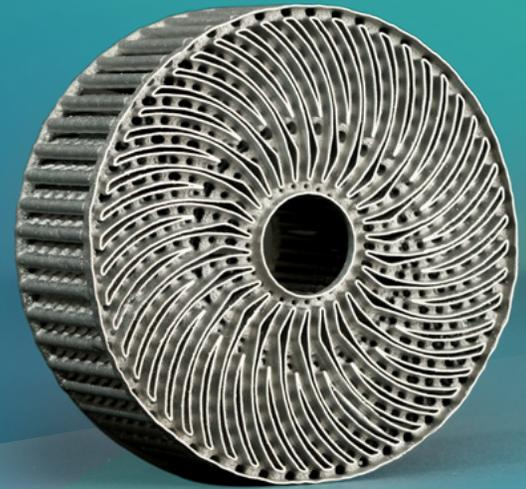
A high precision laser is directed on to metal powder bed, selectively melting and building up thin horizontal metal layers. This technology allows for the production of metal parts with challenging geometries, not possible using traditional subtractive or casting technologies.
