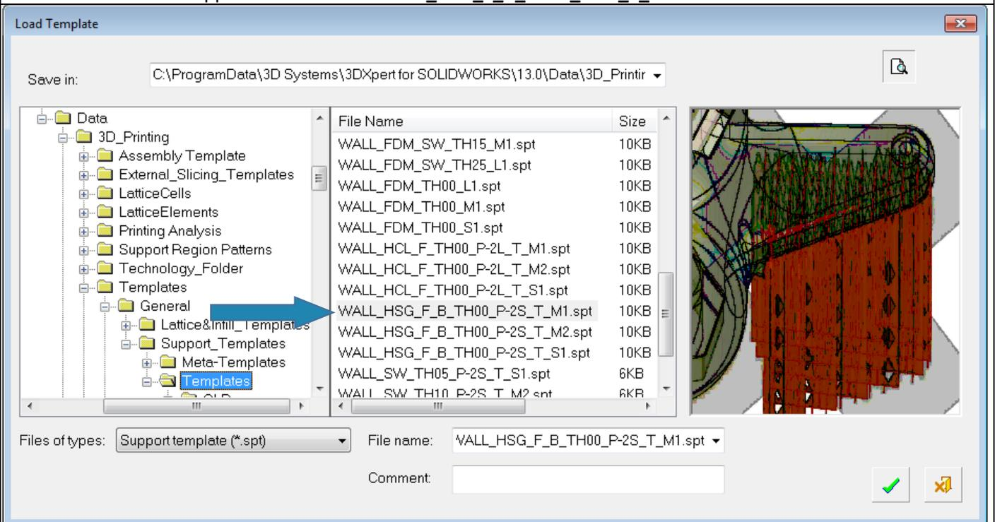
This family of supports can give a very good cover for small up to large regions with a good strength and yet easy to remove due to the "**Teeth**" (**T** in the code name) at the touch points with the part.
