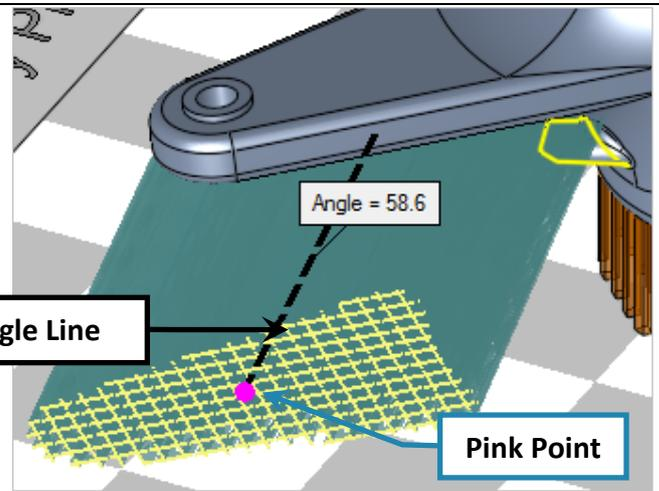
Pick anywhere on the **Angle Line**, a Red Point appear. It is possible to drag it to any direction as well add scaling to the support's section. It is also possible to pick the point at tray level (Pink Point) to move and scale it as well if needed. By doing so, we released the detail so the support won't rely on it on the upper side.
