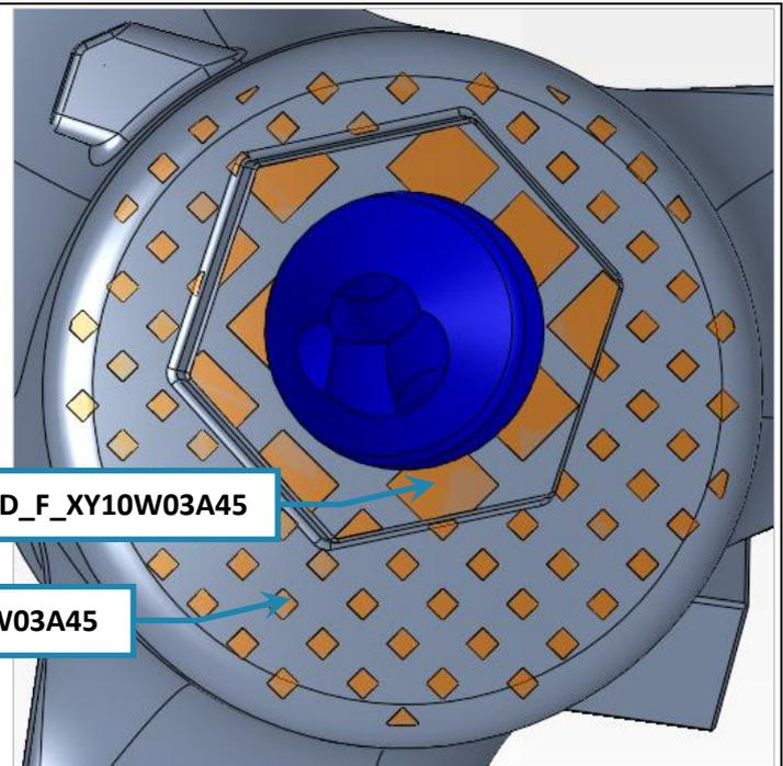
Note on the Table of regions that a bulb was added automatically to indicate that a support was added on this region. The bulb of this region itself is now in **Hide** mode (as this region is no longer required) while the bulb of the relevant support turns to **Show** mode.
