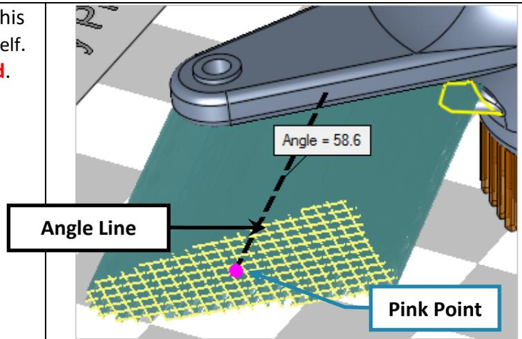
Pick anywhere on the **Angle Line**, a Red Point appear. It is possible to drag it to any direction as well add scaling to the support's section. It is also possible to pick the point at tray level (Pink Point) to move and scale it as well if needed. By doing so, we released the detail so the support won't rely on it on the upper side.
