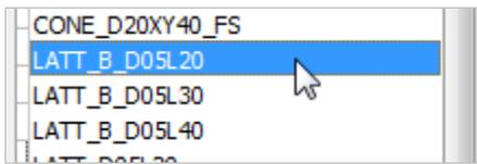
This family of supports can give a very good cover for small medium up to very large regions with a good strength and yet easy to remove because of the **Ball (B** in the code name) shape at touch points with the part.
