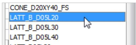
This family of supports can give a very good cover for small medium up to very large regions with a good strength and yet easy to remove because of the **Ball (B in the code name)** shape at touch points with the part.
