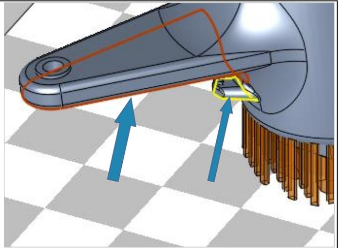
From the **Supports Manager** window **pick Template By Reference**
