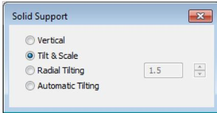
This will allow us to move the support on the tray and if necessary to scale and shrink it so it won't gauge with the part.
