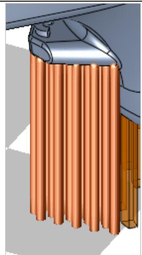
It is also possible to tilt the Cone Support to minimize touching with the side of the part.
