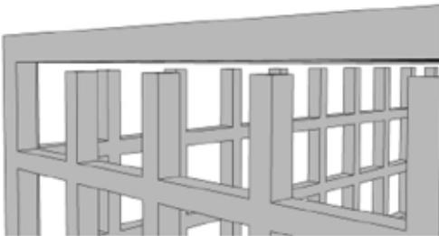
In applications requiring additional post processing, such as sterilization for surgical use, the batch can transition through the various processes within the cage. To remove the parts consider CAD modeling in hinge doors, apply snap-off regions or, as in this example, connect the lid with the four corner posts that can be cut off with wire snips.
