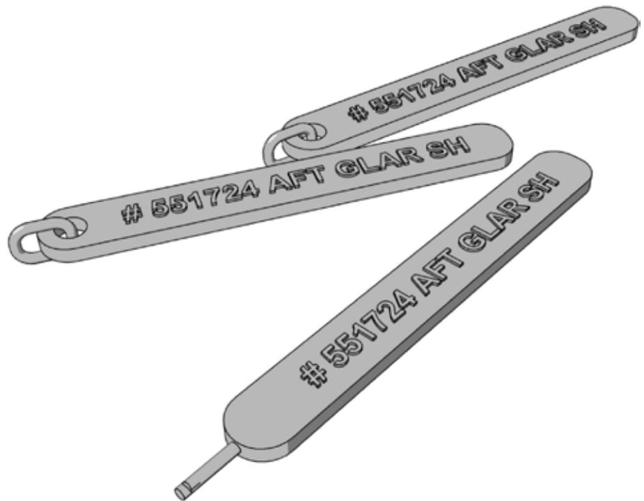
Note in the above stick, to “tag” connector the junction between the stick and the part is in a depressed filleted pocket, this reduces the impact on the mechanical integrity of the part. Also note the snap point in this case, a V notch modeled into the stick. The same can be applied to chains where you want to enable easy controlled removal of the tag.
