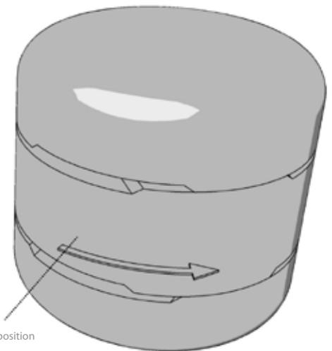
To solve this, one approach is to apply a form where the hinge rotates into a flush position. Generous tolerances in excess of 1mm can be applied in the disengaged state for building, while tolerances of approx 0.05mm will enable a flush intimate stable interaction in the engaged functional range of the rotation.
