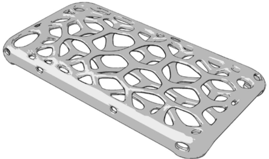
Also note that while you may cut down on the weight of the final part relative to a solid non-grid section, you will increase cleaning time and you will increase draw time on the systems, as the laser now outlines and fills in the feature rich cross-sections.
