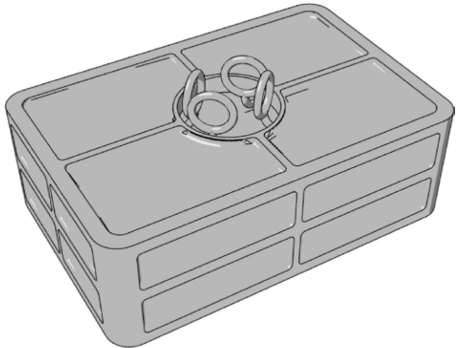
As with #4 air ducts, when designing consider the placement of nested tools and powder removal aids. In this case a combination of rods and chains are used to cut and pull the material cake from the internal corners.
