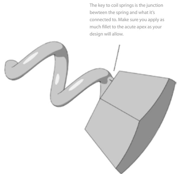
The key to coil springs is the junction between the spring and what it's connected to. Make sure you apply as much fillet to the acute apex as your design will allow.
