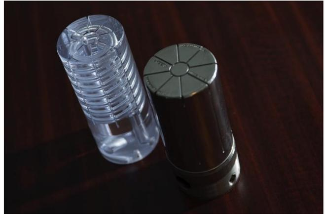
A Bastech mold core insert with conformal cooling channels prototyped using 3D Systems' Stereolithography (SLA) technology and printed in maraging steel on the ProX® DMP 200.
