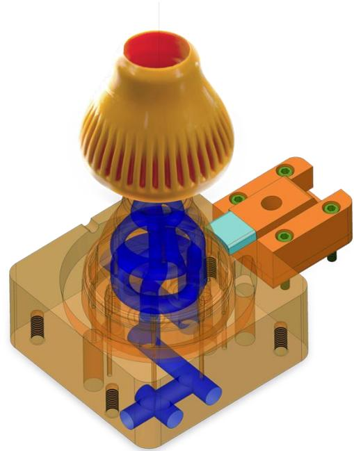
Complex conformal cooling channels created with the comprehensive mold design toolsets of Cimatron™ led to a 14% reduction in cycle time and 16% reduction in overall costs.
