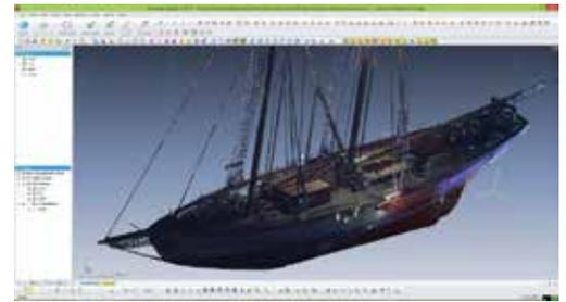
**Image 2: Rendered Point Cloud inside Geomagic Design X**
