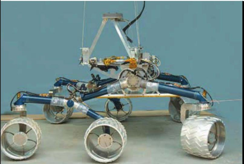
"Scarecrow," a test model for NASA's Mars Science Laboratory, is used to evaluate mobility and suspension performance. Rotor housings sit atop the two-piece, C-shaped strut weldments. Clearly visible above the right-most wheel, both components were produced by Next Intent.
